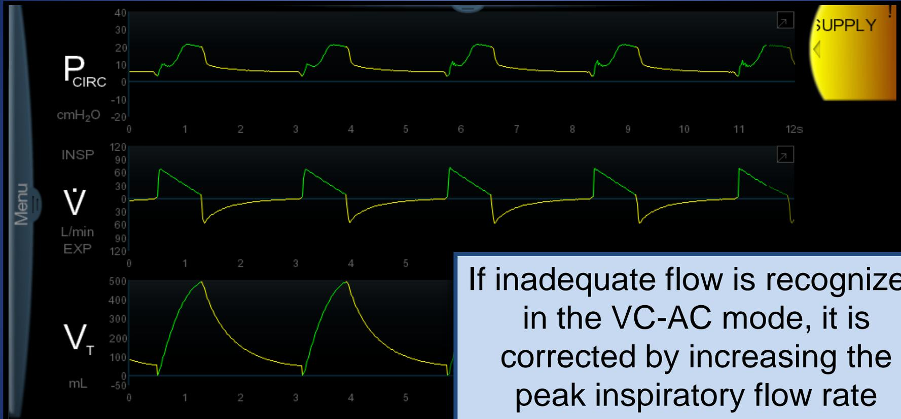
If inadequate flow is recognized in the VC-AC mode, it is corrected by increasing the peak inspiratory flow rate
